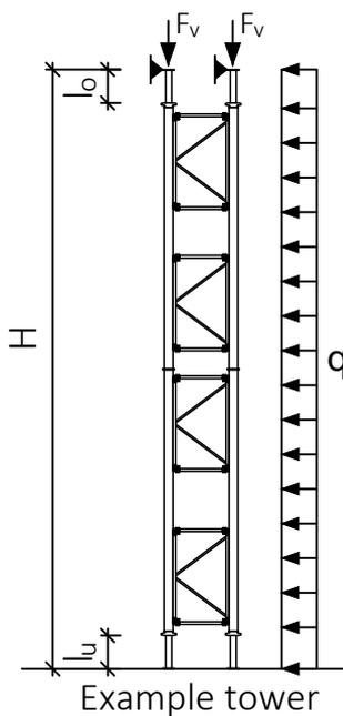
6.2.6 Permissible load for dynamic wind pressure  $q=1.1 \text{ kN/m}^2$  - frame VERTICAL
