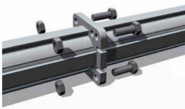
To butt joint two NOEprops, place their end plates together and fasten with 4 M16x40 bolts (Part No. 313400).
