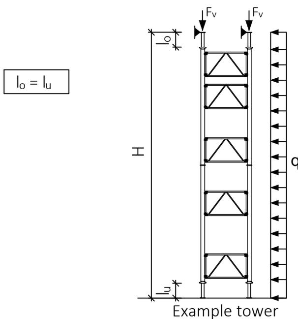
6.2.4 Permissible load for dynamic wind pressure  $q=0.0 \text{ kN/m}^2$  - frame VERTICAL
