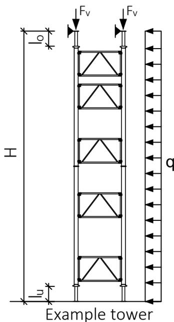
6.2.2 Permissible load for dynamic wind pressure  $q=0.65 \text{ kN/m}^2$  - frame HORIZONTAL
