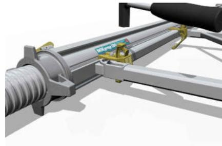
Place the NOEclamp on the corner piece or in the case of a mounted NOEclamp move it into the desired position and engage the clamping jaws in the profile of the NOEprop's external tube.
