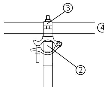
The coupler for the stiffening tube should be attached near the connection point.
