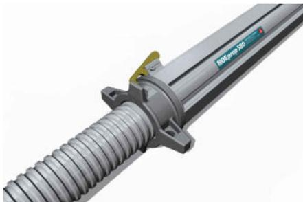
Turn the quick jack nut to finely adjust the prop. To turn the quick jack nut under load use the NOEprop spanner (Part No. 391900).
