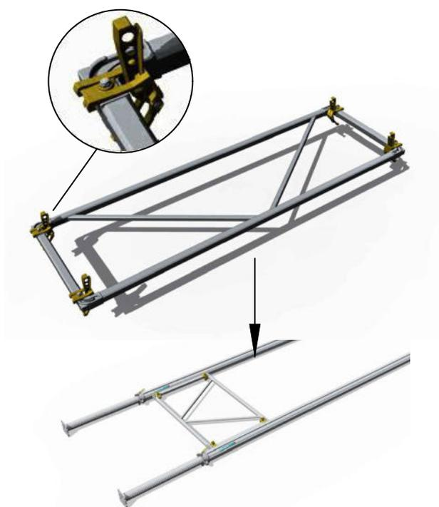
If the frame is used horizontally, then the NOEclamps on the corner piece are placed on the short side of the frame.
