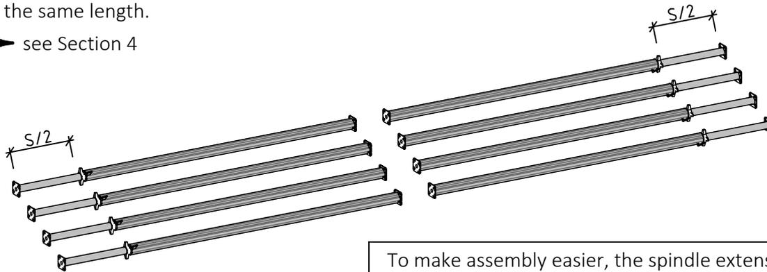
To make assembly easier, the spindle extension on the top NOEprop can be set after the props have been butted together and the frames attached.
