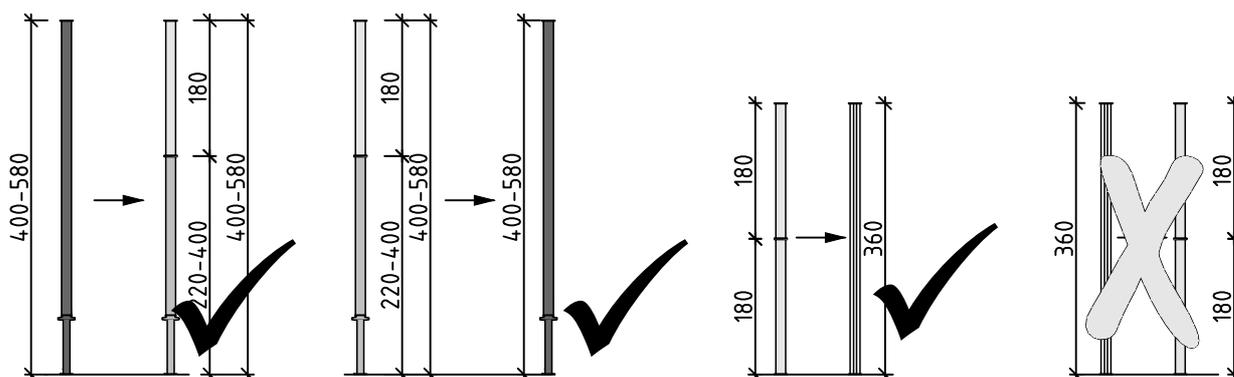
When using the frame vertically, the prop 4.00-5.80 can be replaced by NOEprop 2.20-4.00 and the adapter 1.80 m and vice versa. This also applies to the bottom and top parts.
