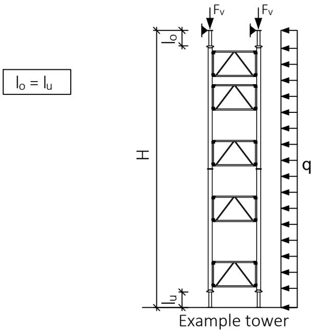
6.2.3 Permissible load for dynamic wind pressure  $q=1.1 \text{ kN/m}^2$  - frame HORIZONTAL
