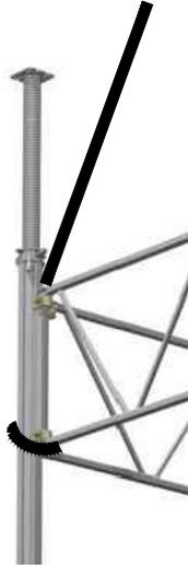
To stand up and transport the tower, the crane suspension must be slung around the NOEprops and the two adjacent top frames.
