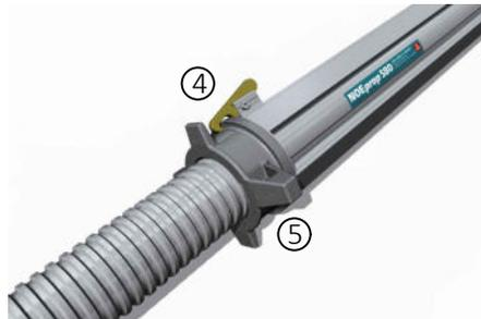
Release the NOEprop hook, it automatically locks the spindle to prevent it being inadvertently screwed out.
