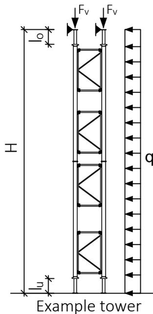
6.2.5 Permissible load for dynamic wind pressure  $q=0.65 \text{ kN/m}^2$  - frame VERTICAL
