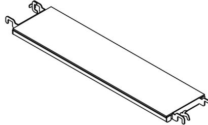
The boarding is designed for a uniformly distributed load of 0.75 kN/m<sup>2</sup> in accordance with EN 12811-1:2001(D).
