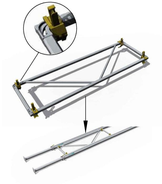
If the frame is used vertically, then NOEclamps on the corner piece are placed on the long side of the frame.
