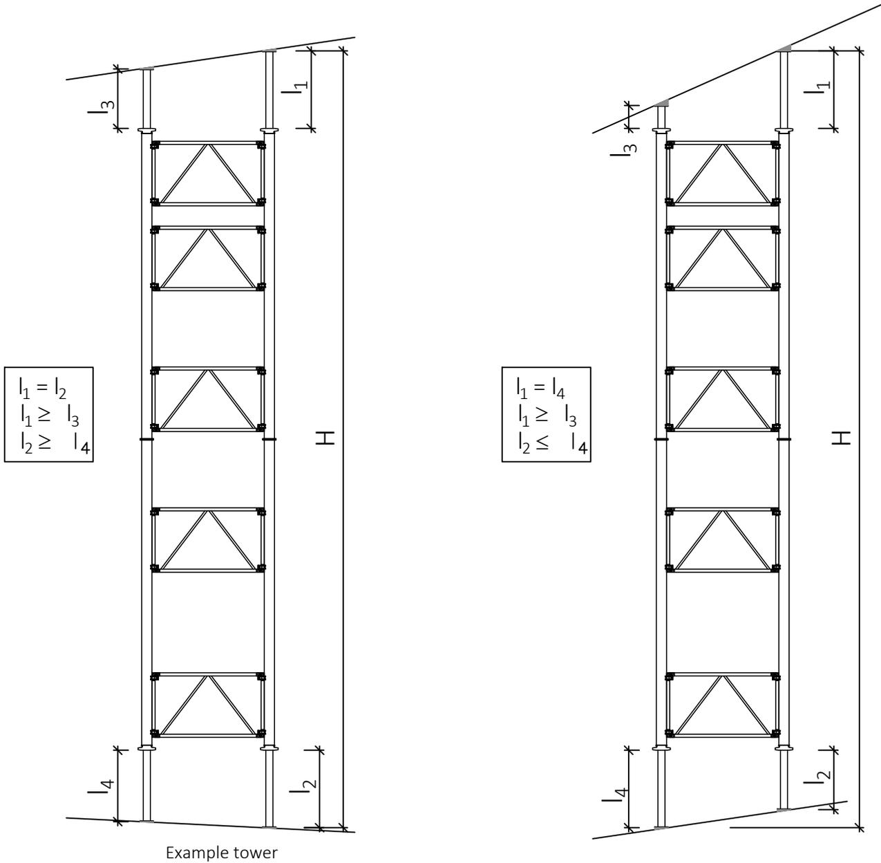
H is the determinant height for reading the permissible vertical load from the load capacity charts.
