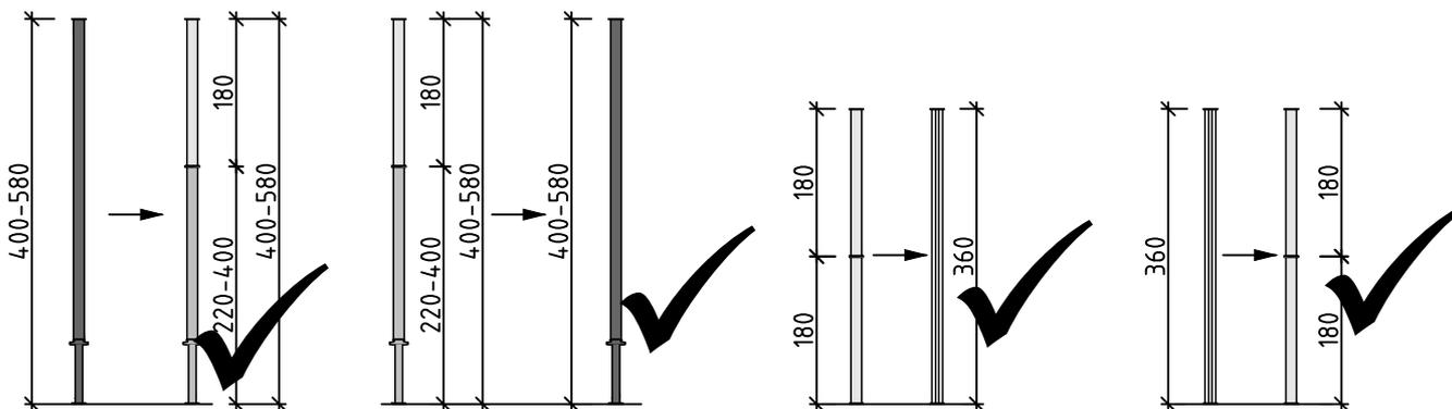
When using the frame horizontally, the prop 4.00-5.80 can be replaced by NOEprop 2.20-4.00 and the adapter 1.80 m and vice versa. This also applies to the bottom and top parts.
