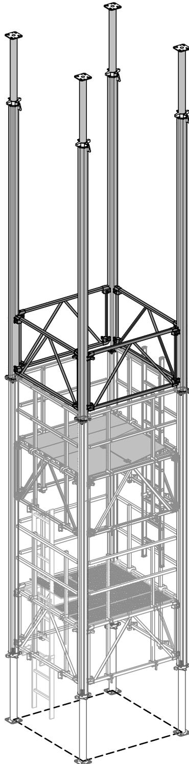
To make assembly easier, the spindle extension can be set after the NOEprops have been butted together and the frames attached. The top and bottom spindle extensions must be of equal length.
