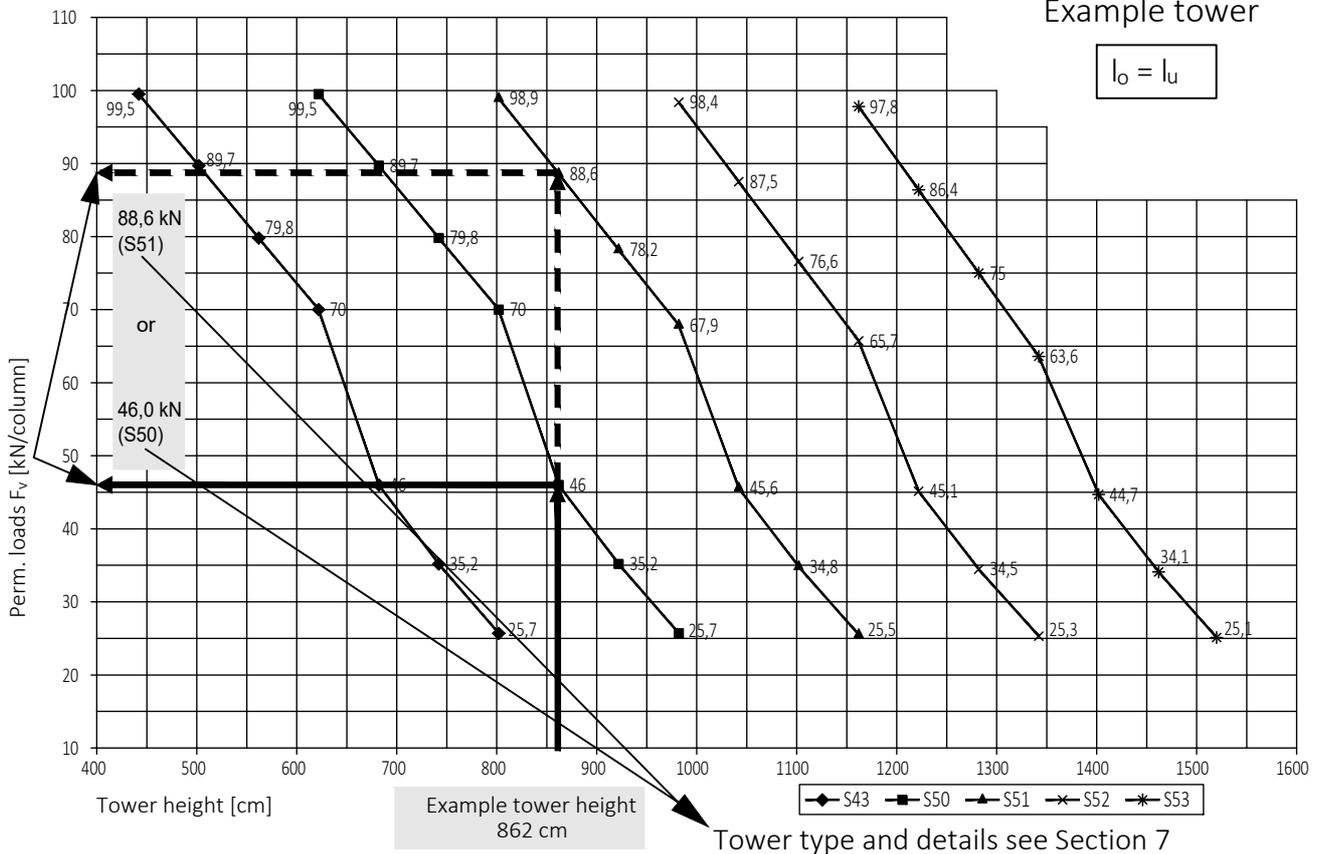
6.2.1 Permissible load for dynamic wind pressure  $q=0.0 \text{ kN/m}^2$  - frame HORIZONTAL
