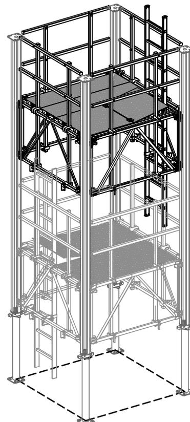
8) Butting on the next props and attaching the next set of frames
